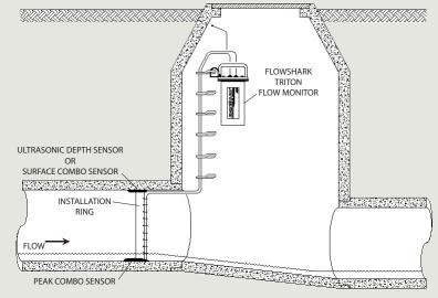
All ADS sensors are mounted within the pipe section where depth and velocity are uniform as the flow passes the sensors. This ensures accurate flow quantification.
